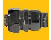
Material: Nickel Plated Brass Temperature Range: -45°C to +105°C continuous Construction: 4 Part Fitting (Body, Metal Ferrule, Sealing Ring & End Cap) IP Rating: IP67
