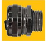
Material: Nickel Plated Brass Temperature Range: -45°C to +105°C continuous Construction: 4 Part Fitting (Body, Metal Ferrule, Sealing Ring & End Cap) IP Rating: IP67
