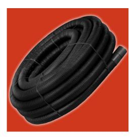
Twin-walled underground burial conduit has a corrugated exterior and a smooth interior core. Manufactured from HDPE by a twin-extrusion process, two pipes are extruded simultaneously (one inside the other) and heatwelded in one continuous process.
